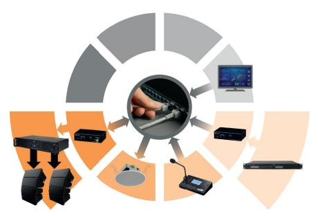
Via HTTP commands, you can change the volume of each IP speaker individually, start and stop music playback, or activate internal messages. The **IP-A1PG** IP paging gateway can distribute analogue audio to various devices in the network simultaneously and provides flexible scheduling options.
